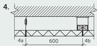
A suspended ceiling system (4a; 5a) or laths construction (4b, 5b) is attached to the ceiling with the „quick“ suspension, then the CEWOOD panels are assembled.
