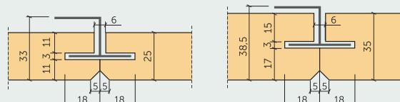
**P5S** - Hidden suspended ceiling profile with overhang and 5 mm chamfer
